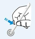
If you press the pen button when the S Pen tip is on the screen, circles appear around the pointer on the screen. Touch the screen with the S Pen while holding down the pen button.
